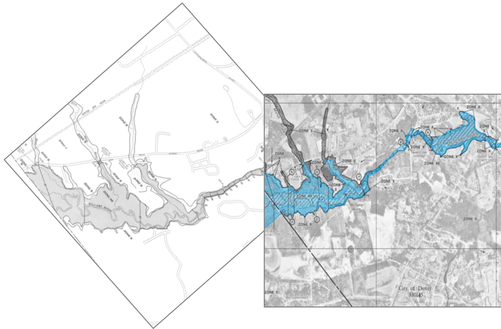
Figure 1. The map on the left is the former Flood Insurance Rate Map for the city of Dover and the map on the right is Dover's current Digital Flood Insurance Rate Map.
