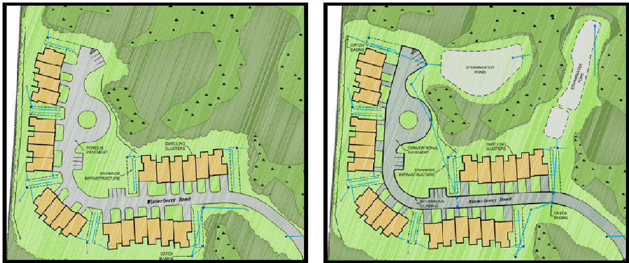
Figure 1: Comparison of Two Designs, LID Design (left) and Conventional (right) for Boulder Hills, Pelham, NH
