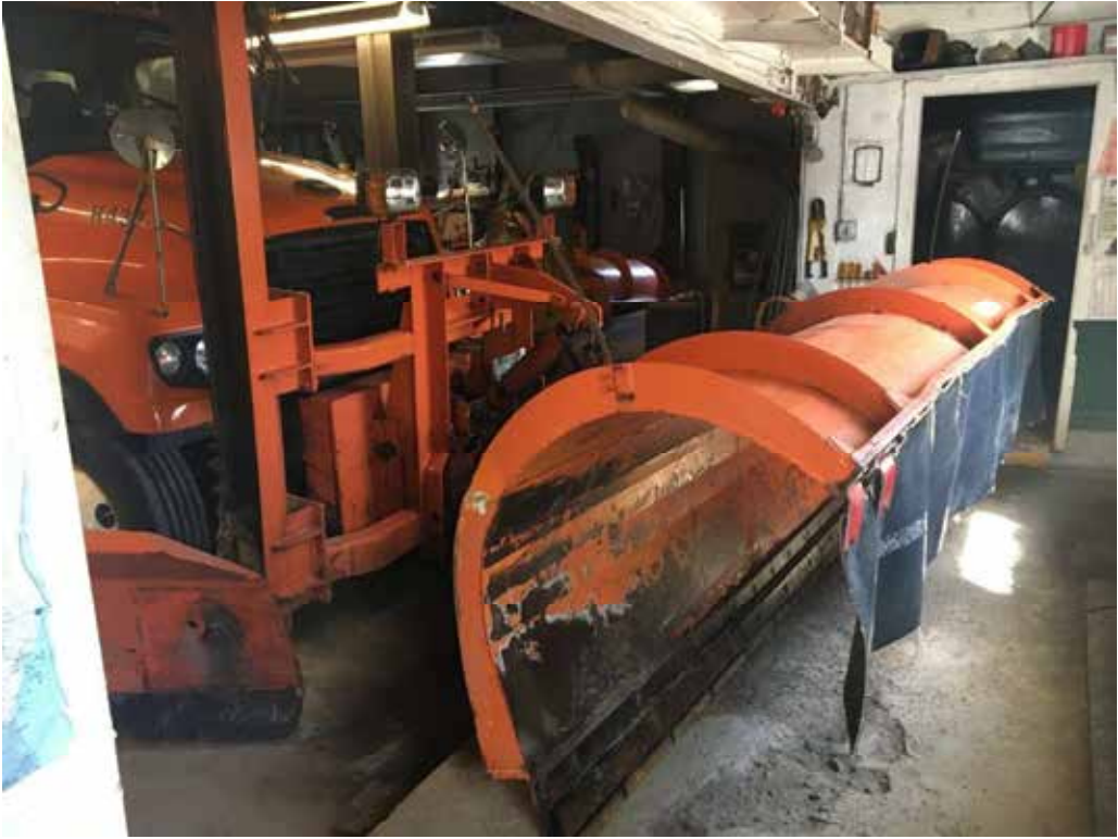
Photo-3: View of the front of truck with plow equipment mounted and parked in shed. Minimal clearances and uneven surfaces throughout the building make it difficult to navigate and increase risk of accidents and injuries.
